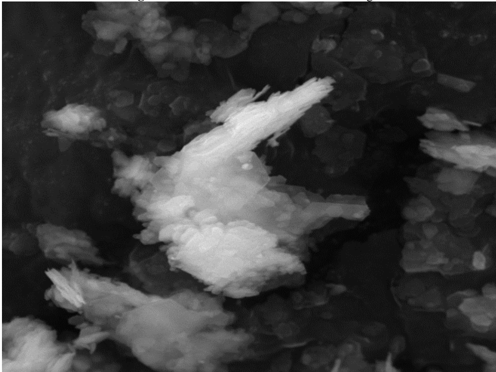
Figura 8 - MEV do material do caulim coating
