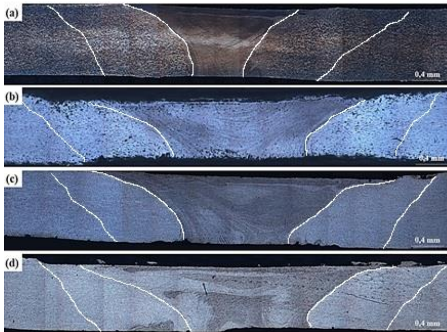
Figura 24: Macroestrutura das amostras: (a) 0 mm, (b) 0,5 mm, (c) 1,0 mm, (d) 2,0 mm.
