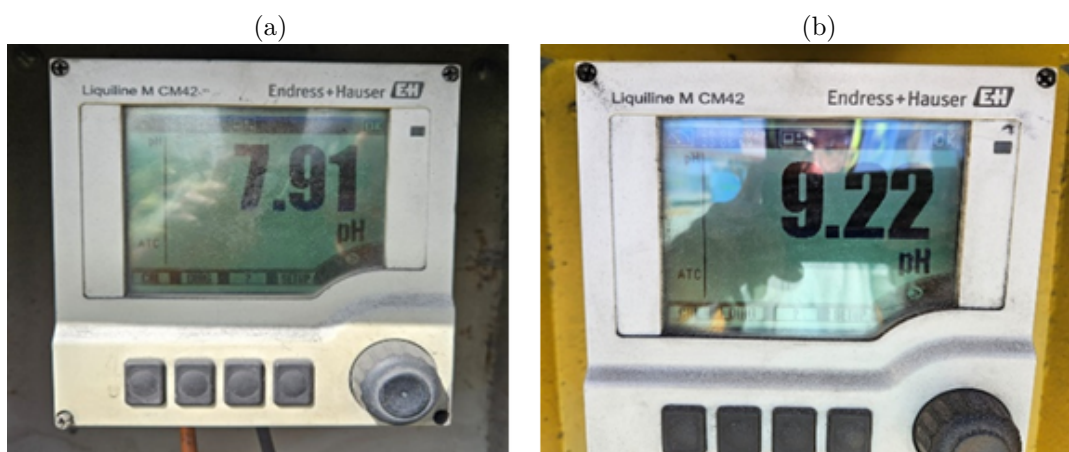
Figura 3 – Sensor de pH do modelo Liquiline M CM42 da Endress+Hauser : (a) pH 7,91; (b) pH 9,22
