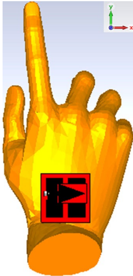
Figure 14. WBAN antenna simulation in human model in CST Studio [11].
